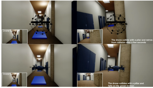
Fig. 6. Simulated test videos. Elios's collision is on the top row and Mavic's collision is on the bottom row.
